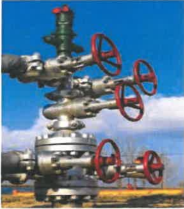
Natural gas wellhead.
